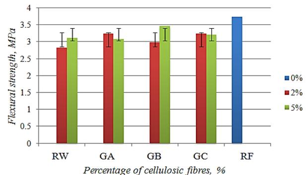
**Fig. 3.** Effect of cellulosic fibre content on the flexural strength of cement mortar specimens
