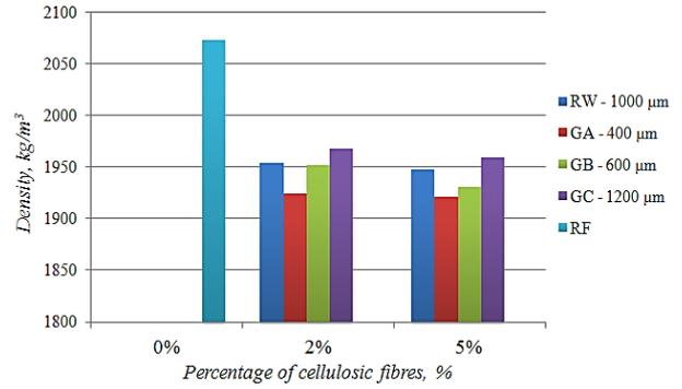
**Fig. 2.** Density of fibre-cement mortars with 2 % and 5 % of cellulosic fibre contents
