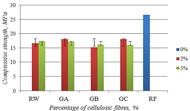
**Fig. 4.** Effect of cellulosic fibres content on the compressive strength of cement mortar specimens
